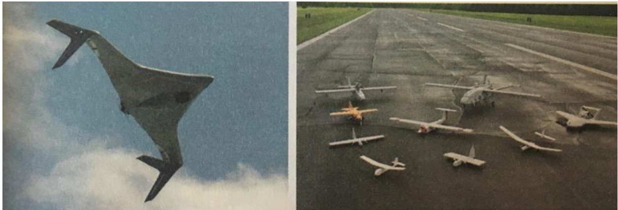
Figure 7 left: Gruman 's UAV carries EO / IR and SAR sensors, laser rangefinder, laser marker and infrared (IR) cameras, right: exhibition of American UAVs in 2005.
