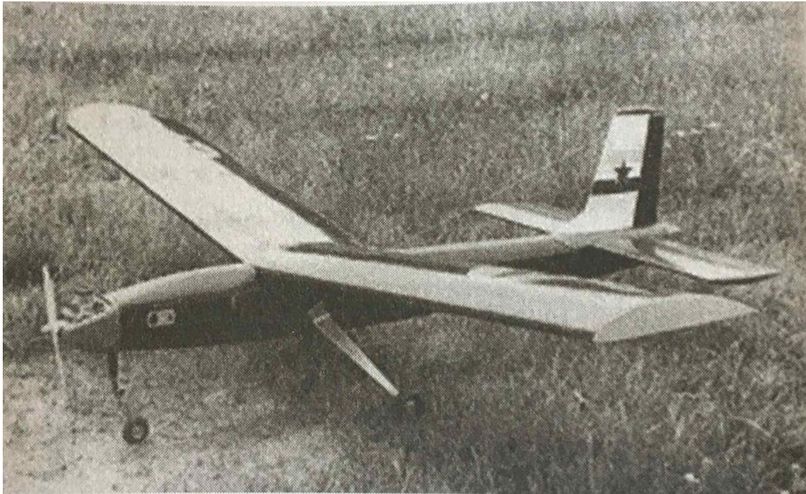
Figure 1: Yugoslav People's Army (YPA) air defense training aircraft with radio control (RC)
