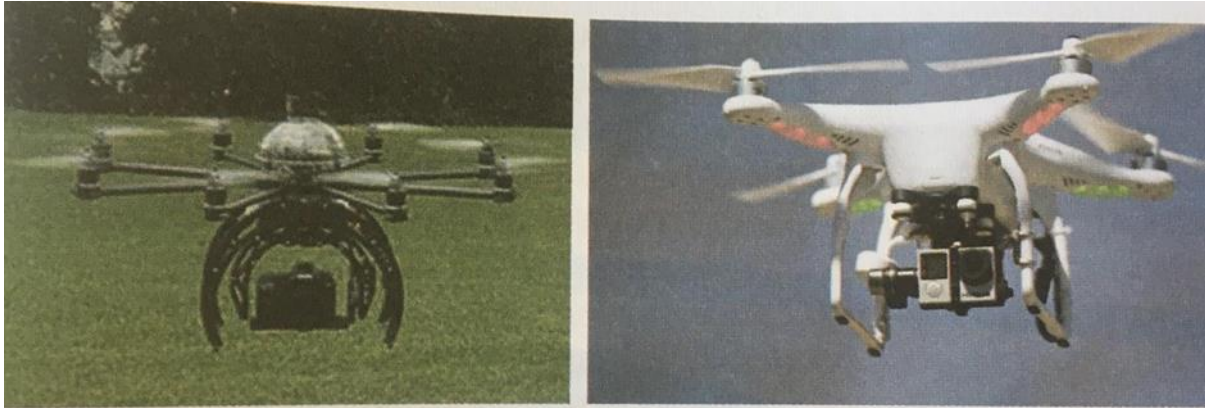
Figure 109. UAV with eight rotors; Commercial UAV (quadcopter, is equipped with a camera product of Chinese by DJI)
