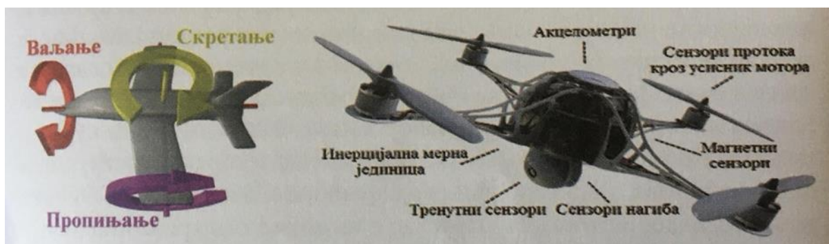
Figure 37. View of the freedoms of movement along and rotation about the three axes of the aircraft
