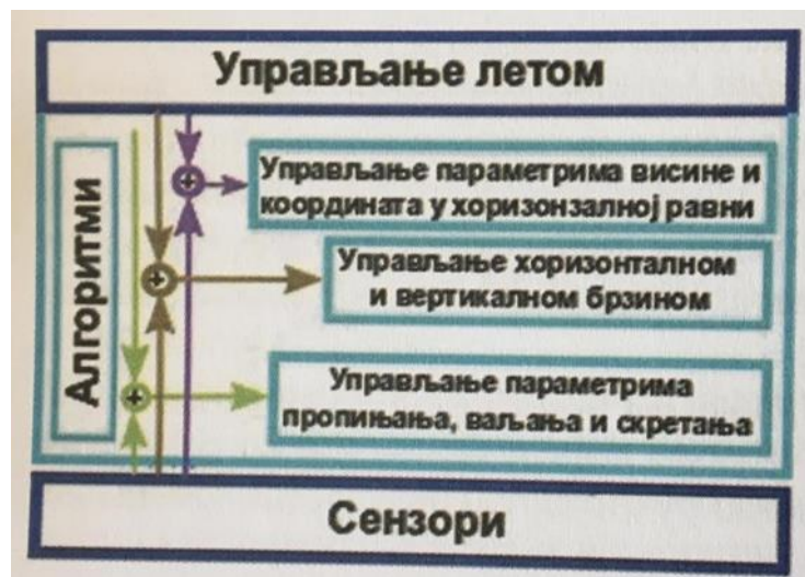
Figure 65. Typical scheme of UAV autopilot flight control
